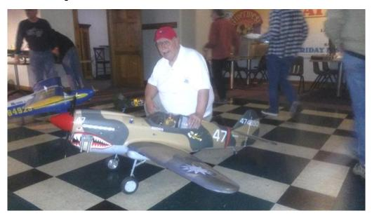
Chris Milbauer brought a Top Flite P40 War Hawk with 86 inch wingspan and powered by a Zenoha G62 gas engine with a Bennett muffler. Chris said he installed a Futaba 14 channel receiver and Hitec servos. The plane has a Beila 3-blade 20 x 10 prop and Dave brown spinner. It is also equipped with Robart electric rotating retracts, a 3600 mAh Life battery for the gear, and a 2100 mAh Life battery for the receiver. The pilot is from Best Pilot.
